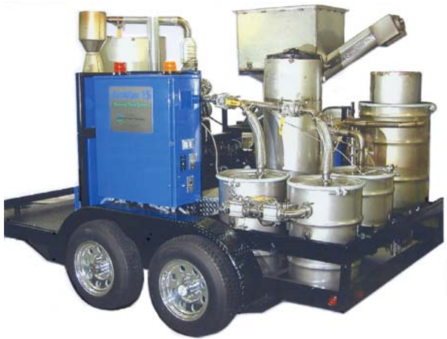
Figure 4. The BioMax 15 is a transportable and fully automated biopower unit that uses wood residues to produce electricity and heat for small enterprises, rural homes, and schools. Still in a pre-commercial development stage, units are now being tested at seven sites around the United States, including White Spruce Enterprises in Salcha, Alaska; Mount Wachusett Community College in Gardner, Massachusetts; and SBS Wood Shavings in Glencoe, New Mexico. Photo courtesy of Community Power Corporation, Littleton, Colorado
