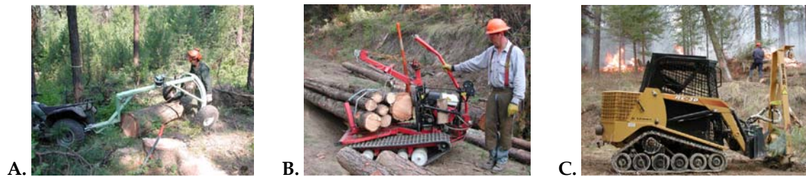
Figure 1. Basic harvesting technology equipment used in Halbrook (2004): A.) ATV with skidding arch, B.) Iron Horse skidding machine, C.) ASV with extraction winch. Photos courtesy of Jeff Halbrook.
