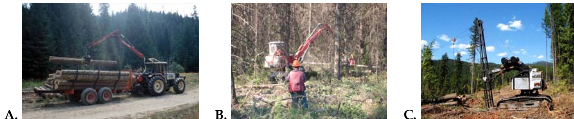
Figure 2. Modified and purpose-built equipment harvesting equipment. A.) Farm tractor base, equipment with a forwarding trailer, B.) Neuson 1002 HV, small scale tracked harvester, C.) Modified tracked feller-buncher for skyline yarding. Photos courtesy of Han-Sup Han.
