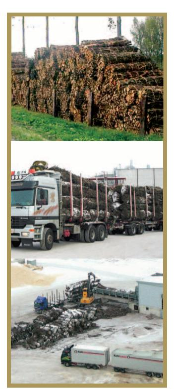
Thanks to compression and bundling, slash can be transported out of the forest with normal forwarders or log lorries. The slash logs can be delivered directly to a power plant or stored temporarily in the forest. The latest communication technology ensures efficient logistics and fast data transfer.
