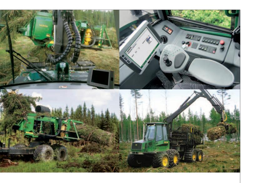
The 1490D collects the slash and residual left behind after harvesting and feeds it into the bundler, which compacts slash into compact logs. The bundling process is continuous, with no restrictions on the length or type of material bundled.
