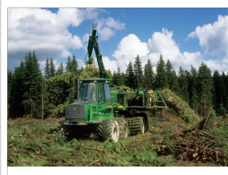
The John Deere 1490D Slash Bundler collects, compacts, and wraps the slash into bundles that can then be easily transported.
